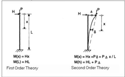
According to the EC-EN 1999, 1<sup>st</sup> Order analysis may be used for a structure, if the increase of the relevant internal forces or moments or any other change of structural behaviour caused by deformations can be neglected. This condition may be assumed to be fulfilled, if the following criterion is satisfied:
