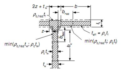
The section properties are then recalculated based on the reduced thicknesses.
