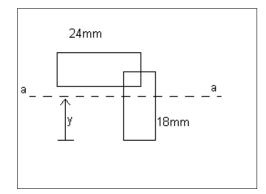
$b_{eff}$  = For RUO reinforcement taken as 12xt t = 2mm
