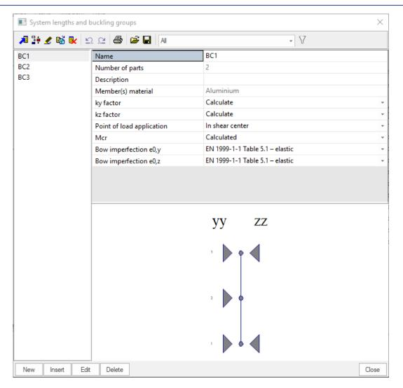
On the left part a list is presented of the defined buckling groups within the project. The list allows multi selection which enables the user to modify common settings at once in that dialog.
