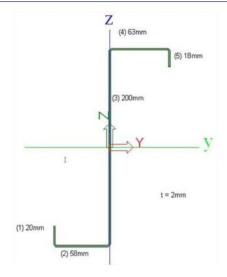
The material properties are as indicated in EC-EN1999: EN-AW 6082 (Sheet) T61/T6151 (0- 12.5):  $f_0 = 205 \text{ N/mm}^2$ ,  $f_{0,HAZ} = 125 \text{ N/mm}^2$  $f_u = 280 \text{ N/mm}^2$ ,  $f_{u,HAZ} = 280 \text{ N/mm}^2$ Buckling curve: a Fabrication: welded
