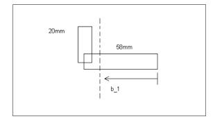
$$b_1 = \frac{(58 \times 2) \times \frac{58}{2} + (20 \times 2) \times 58}{(58 \times 2) + (20 \times 2)} = 36,44 \, mm$$
