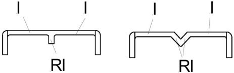
RUO: The reinforcement is connected to only one plate with type I.
