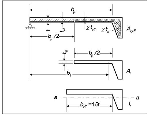
Step 3: Calculation of stiffener buckling load
