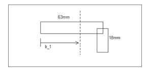
$$b_1 = \frac{\frac{(63 \times 2) \times \frac{63}{2} + (18 \times 2) \times 63}{(63 \times 2) + (18 \times 2)} = 38,5mm$$
